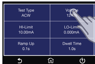
TAP TEST SETTING Tap the test parameter you would like to edit. Swipe up and down to scroll through test parameters.
