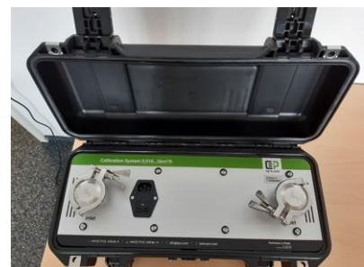
1 Mobile measuring box with integrated gas meter for use on site
