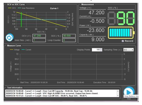
Measurement: Real-time display of electrical performance parameters and SOC status of the existing simulated battery. During the test process, click "Record" to record the existing test data in the CSV file under report file
