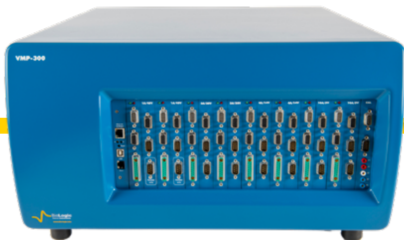
VMP-300 16 channels, \pm 150 A down to 100 fA
