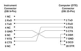
Figure 8 Serial Cable Wiring
