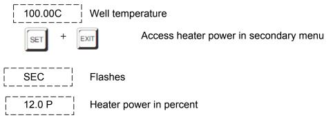
To exit out of the secondary menu hold "EXIT". To continue on to the proportional band setting function press "EXIT" momentarily or "SET".
