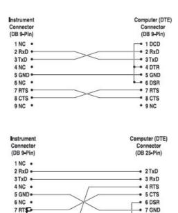
Figure 8. Serial Cable Wiring
