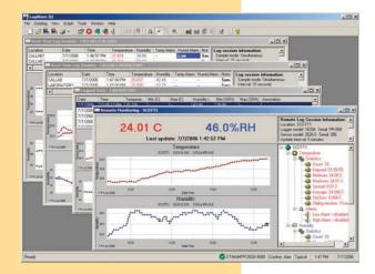
plained can be highlighted, annotated, and referred to later. LogWare III statistics include min, max, spread, average, and standard deviation functions, and printed reports keep track of the number of temperature and humidity measurements that were found to be out of tolerance.
