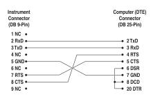
Figure 9 Serial Cable Wiring
