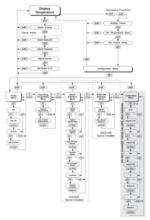
Figure 7 Controller Operation Flow Chart
