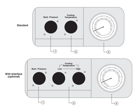
Figure 3 Refrigeration Side Panel Controls
