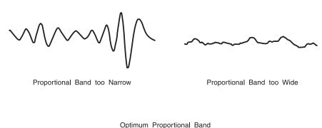
Figure 6 Bath temperature fluctuation at various proportional band settings
