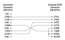
Figure 7 Serial Communications Cable Wiring
