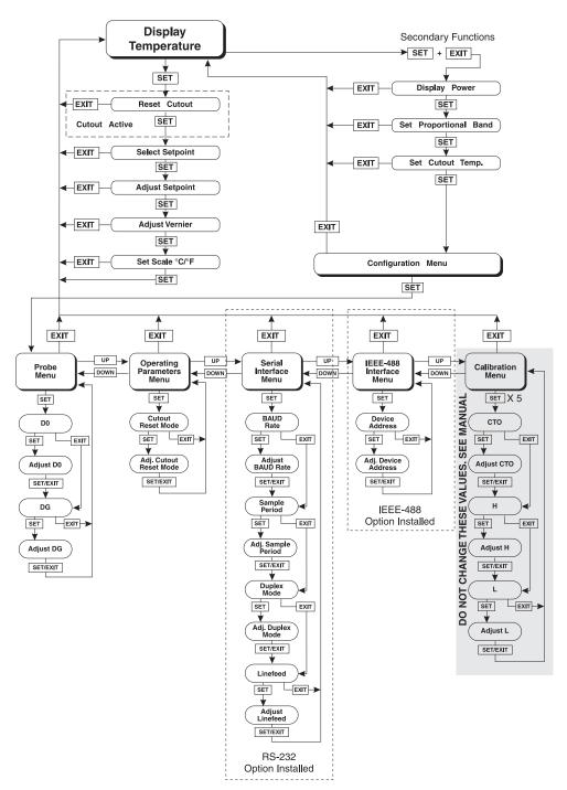
Figure 5 Controller Operation Flowchart
