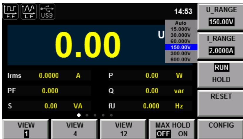
Figure: Voltage Range(Take IT9121 as an example, see the following figure.)
