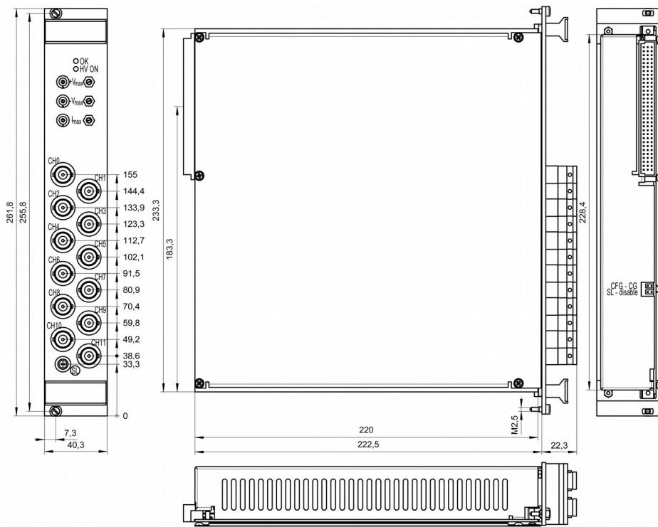
Figure 2: dimensional drawing 6U SHV
