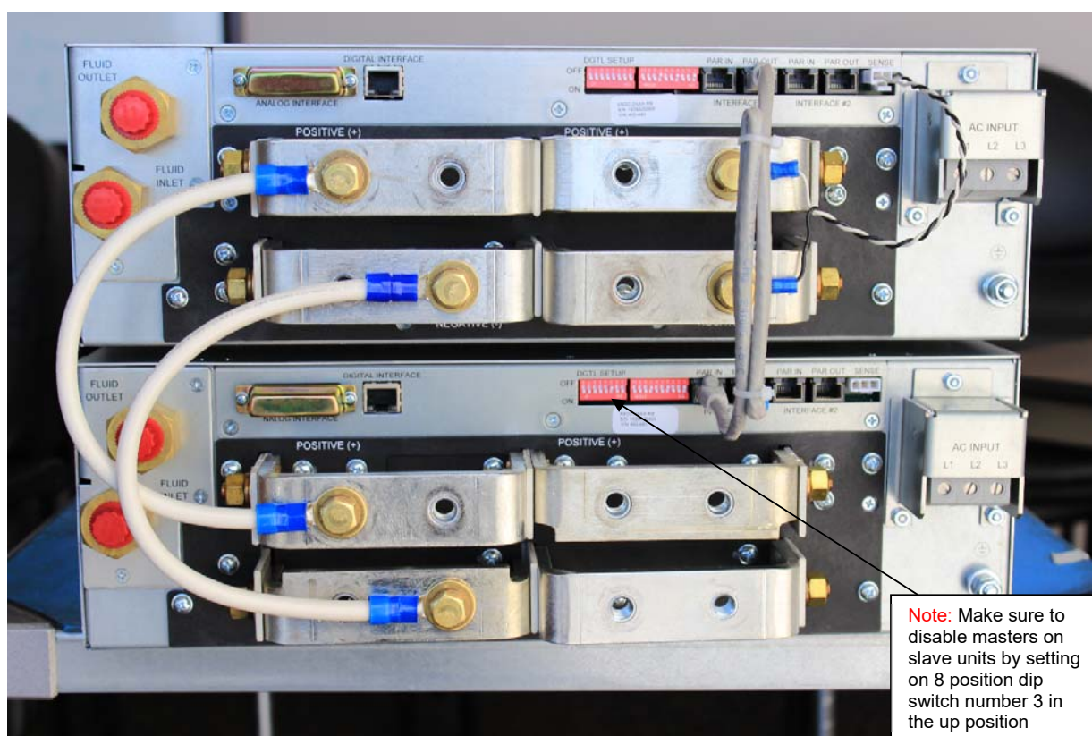
Figure 3-11. Parallel and Remote/Local Sense Connections
